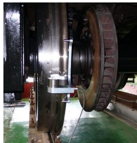
Fig. 2. Wheel profile gage.
